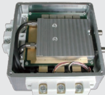
SiC-QMET, motor (left) and AC drive (right) for electric vehicles employing a next-generation SiC semiconductor device
