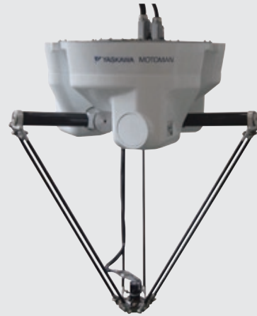
Delta Robot for high-speed material handling MOTOMAN-MPP3
