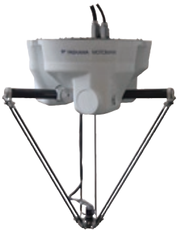
Delta Robot for High-speed Material Handling MOTOMAN-MPP3
