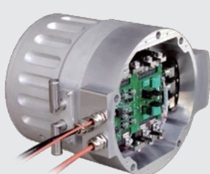
SiC-QMET, motor (left) and AC drive (right) for electric vehicles employing a next-generation SiC semiconductor device
