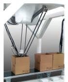
Robot Caser (Box Packing Machine)
