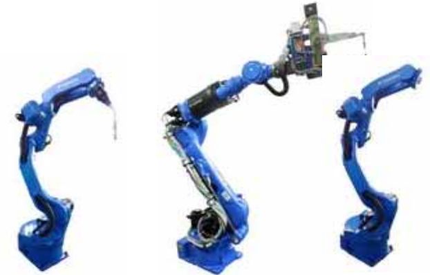
Arc welding robot
