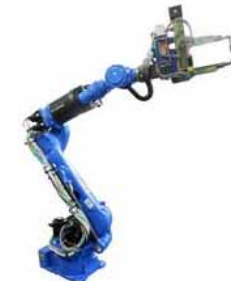
Spot welding robot
