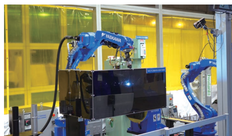
Demonstration of EAGL method in which the amount of spatter in arc welding is significantly reduced
