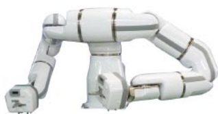
Dual-arm robot for biomedical uses MOTOMAN-BMDA3 (Several patents, specialized to the biomedical business, are pending.)
