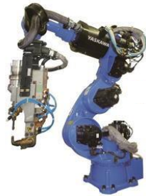
New spot-welding robot with 7 axes
