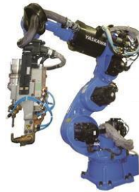
New spot-welding robot with 7 axes
