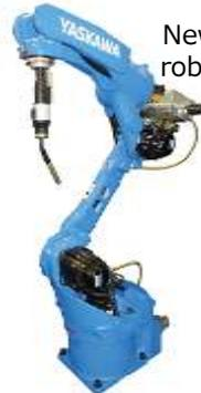
New spot-welding robot with 7 axes
