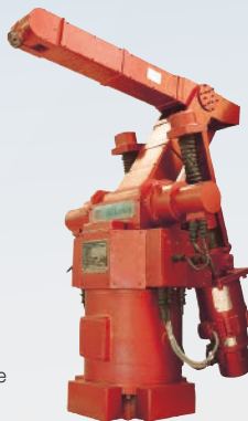
MOTOMAN-L10 Japan's first all-electric articulated robot
