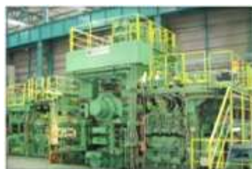
Cold rolling mill
