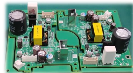
A substrate for servo amplifiers made in YASKAWA (Changzhou) Mechatronics system Co., Ltd.
