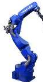
7-axis arc-welding robot MOTOMAN-AR1440E
