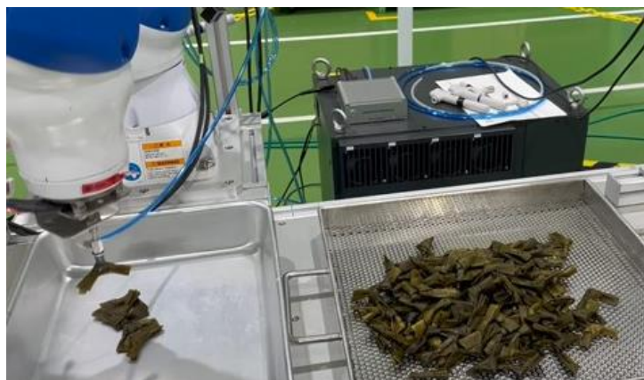
Robot that uses AI to accurately pick “knot” of knotted kelp
