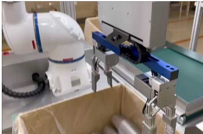
Robot that uses AI to take out cups stacked in cardboard boxes
