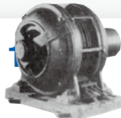
20HP three-phase induction motor (1917) Yaskawa's first commercial product
