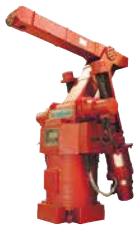
MOTOMAN-L10 (1977) Japan's first all-electric vertical articulated industrial robot
