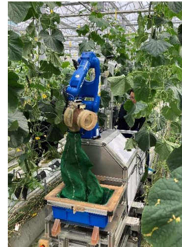
Cucumber leaf-removing and harvesting robot currently operating at Yume Farm ZEN-NOH SAGA
