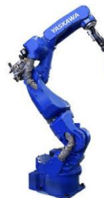
7-axis arc-welding robot MOTOMAN-AR1440E
