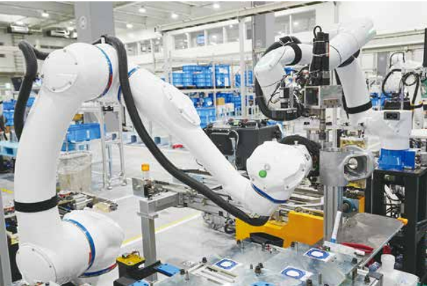
Autonomous AI robot “MOTOMAN NEXT (NHC12)” performing screw-fastening operations
