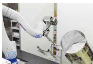
Acquire depth images with a vision camera
