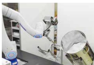
Acquire depth images with a vision camera
