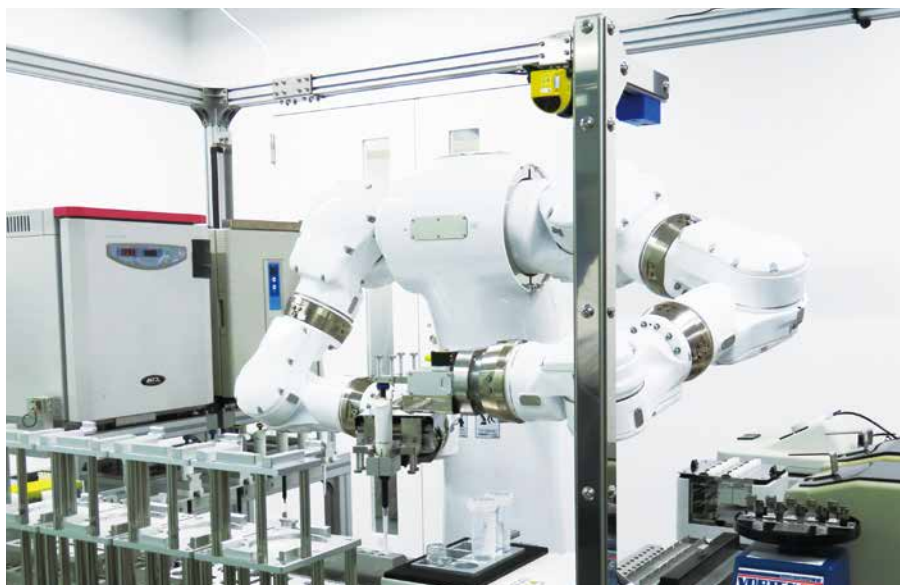
General-purpose humanoid robot LabDroid "Maholo" operating on a cell manufacturing platform
