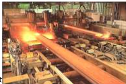
Continuous casting equipment
