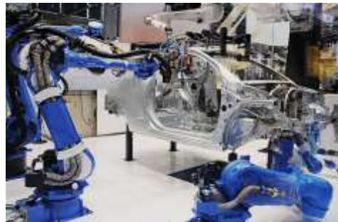
Car production line spot welding system
