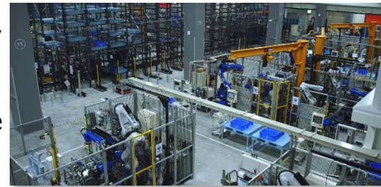
Robot production at the Factory No.5 utilizing a decentralized cell manufacturing system
